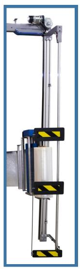
High visibility with ultra-sensitive capabilities to detect barriers in its pathway, from floor to top of the load.
