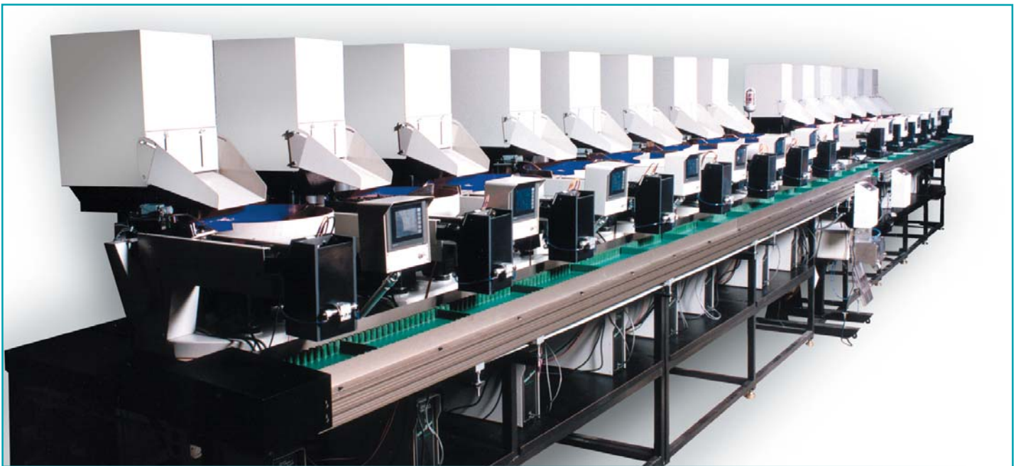
Multi-bowl parts counter for bagging swing set hardware/fastener kits
