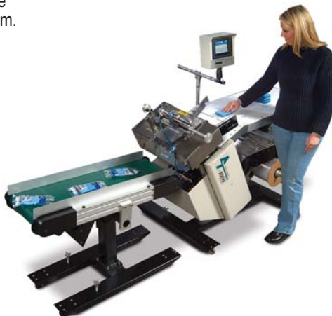
Bulky or lightweight products are difficult to package in a traditional, vertical bagger. Davida manually slides product (spongest) toward an open bag.
