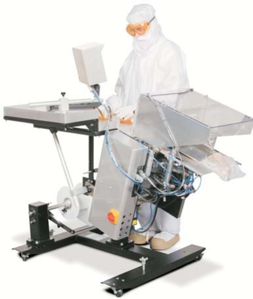
Kyle is using a custom stainless steel loading shelf to package products in a medical clean room.
