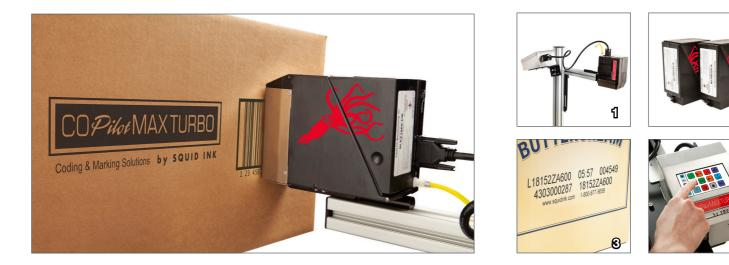
**1)** CoPilot Max Turbo's revolutionary active ink system allows conversion to downshooter mode in seconds.
