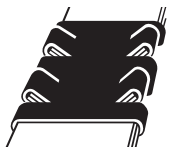
Reverse notch joint
